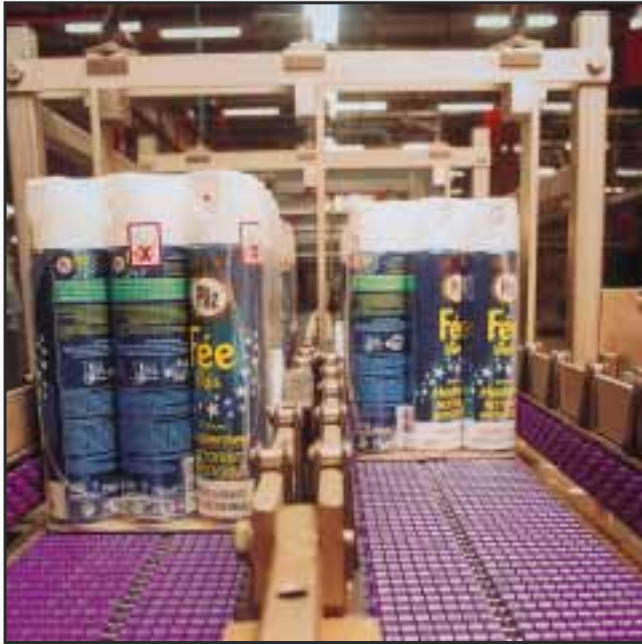
SMOOTH MULTI-PACK CONVEYOR WITH PLASTIC LBP CHAIN.
