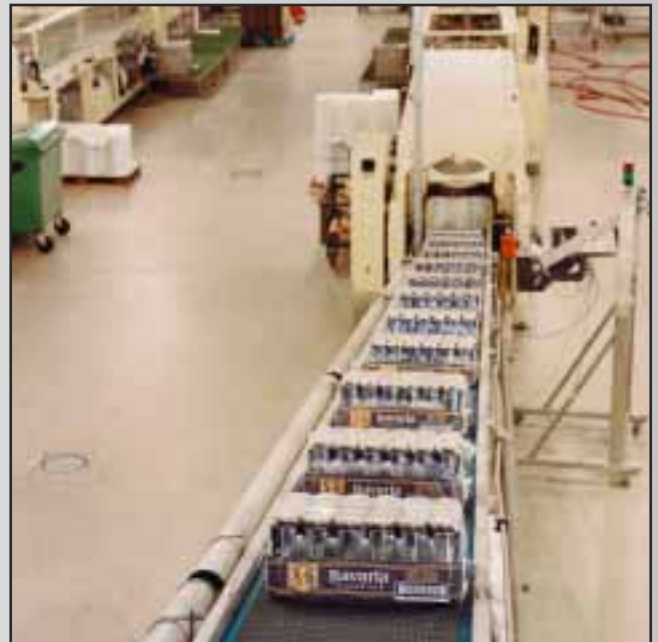
HEAVY TRAYS ON SIDE-INDENT 1005 SUPERGRIP BELT.
