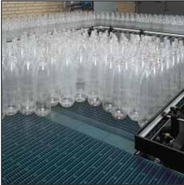
SMOOTH BOTTLE TRANSFER WITH PLASTIC CLICK-COMB FINGERPLATES.
