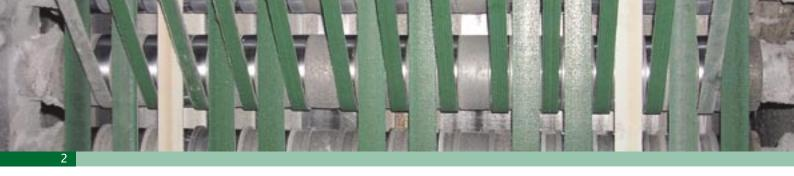
Machine tapes, conveyor and folder belts for paper and printing industry
