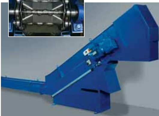
■ Hinged belt conveyor developed for the Trumpf TUBEMATIC laser cutting machine. Special hinged belt plates prevent jamming of the material to be conveyed.
