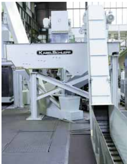
■ Hinged belt conveyor for loading of a hopper system
