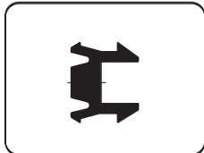
Part. S0370 - Pag. S74 Sealing profile for Part.422. Improves Guide cleanliness.
