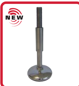
Part. R0752S - Pag. R48 Ø 120 • Stainless steel • Hygiene • Max. load 50000 N.
